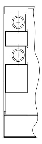
STEP 1: REMOVE SKIN AROUND THE COLLAR, UNTIL THE NEXT **END POST OR STRINGER EXTENSION IS EXPOSED**
