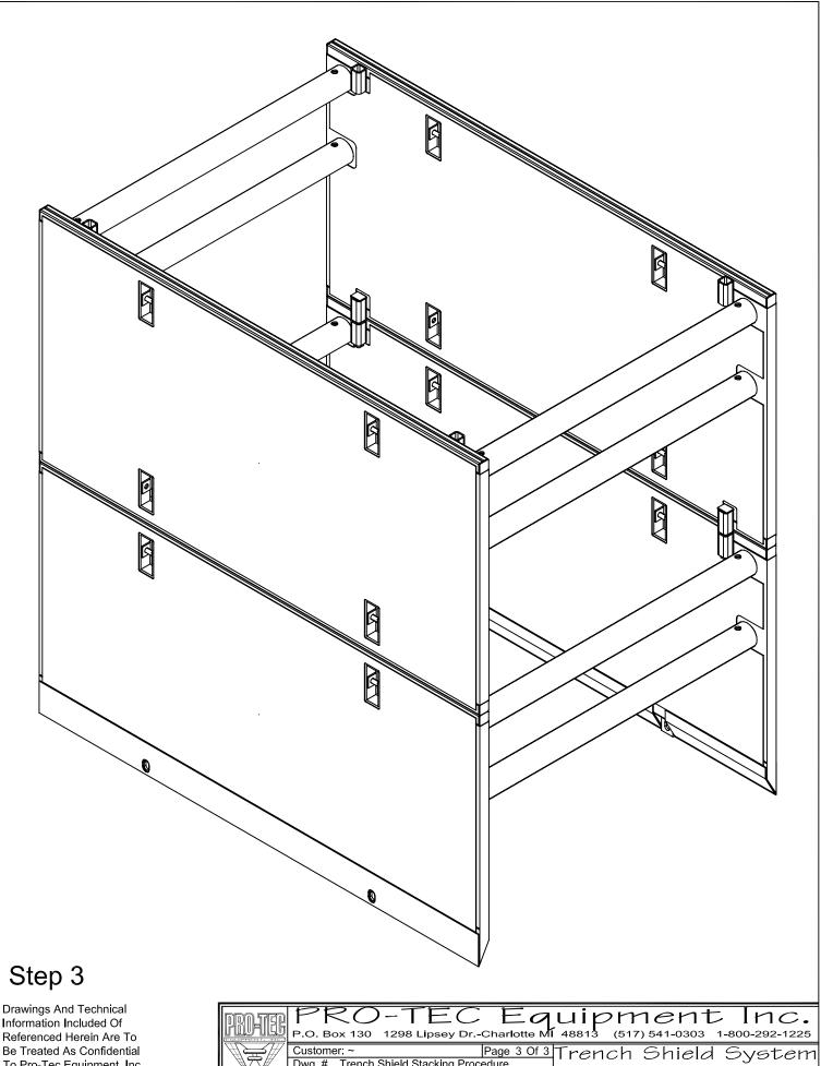
Dwg # Trench Shield Stacking Procedure
